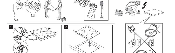
After the electrical connection (see the chapter "Electrical connection"). Position each fixing clips on the dedicated slots on the lateral sides of the hob as shown in the picture. Then push the hob inside the cut out and check that the glass is flat and parallel to the worktop. The fixing clips are designed for every type of worktop material (wood, marble, etc).
